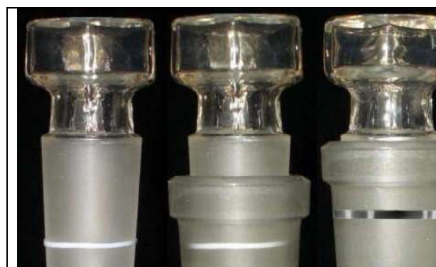
Figure 1. Left: PTFE-sealing ring fixed elastic (no groove necessary). Middle: Sealing ring intransparent without pressure. Right: Sealing ring transparent under sealing pressure.
